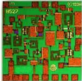
21-34 GHz Downconverter MMIC 1,2x1,2 mm 2
